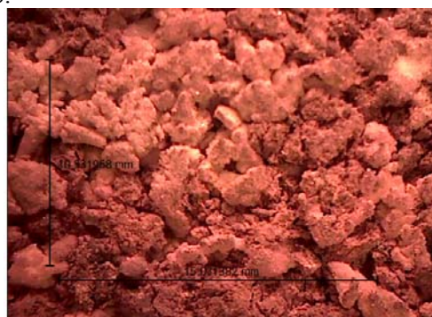
Fig. 1. A structure of porous material based on titanium and saponite
