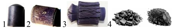
Fig. 2 Changes in the morphology of the sample, depending on the time of exposure to radiant energy at the 900 - 1000 °C: 1 – initial sample; 2 - 1 hour; 3 - 3.5 hours; 4 - 6 h exposure; 5 – form of final products of sample oxidation after grinding in a mortar
