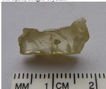
Fig. 1 Photo of a piece of the \text{TlPb}_2\text{Br}_5 single crystal used in the present experimental studies
